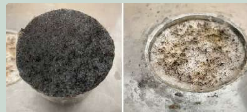
Fig. 1 High adhesion to concrete test - DIN EN 1348
